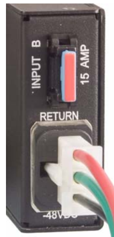
Figure 3. ATCA-6002 INPUT B with keyed power connector in place
